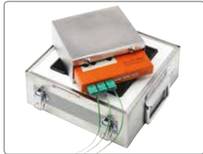
High Temperature Barrier Kit Thermal barrier & heat sinks for longer time at temperature
