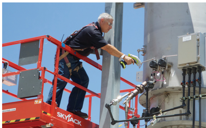
A technician performs positive material identification on pressure vessel components using the Thermo Scientific Niton XL5 Plus analyzer.
