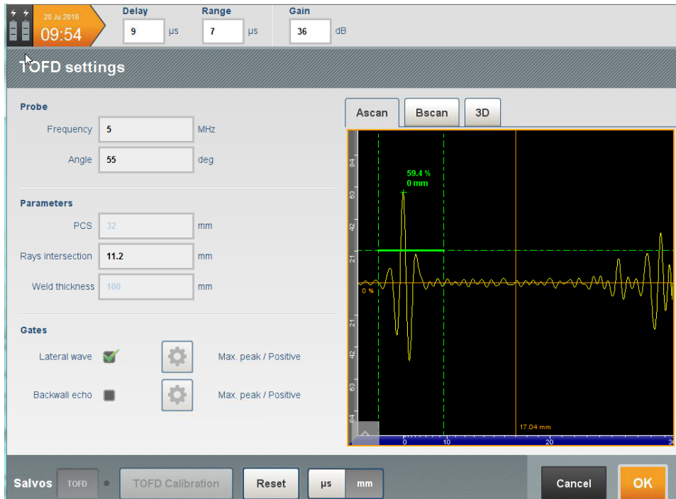
Figure 138: TOFD Calibration (Lateral wave and PCS)
